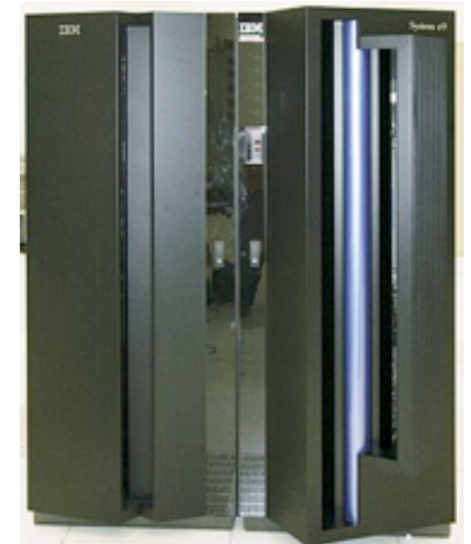
Main Frame (IBM system z9)
